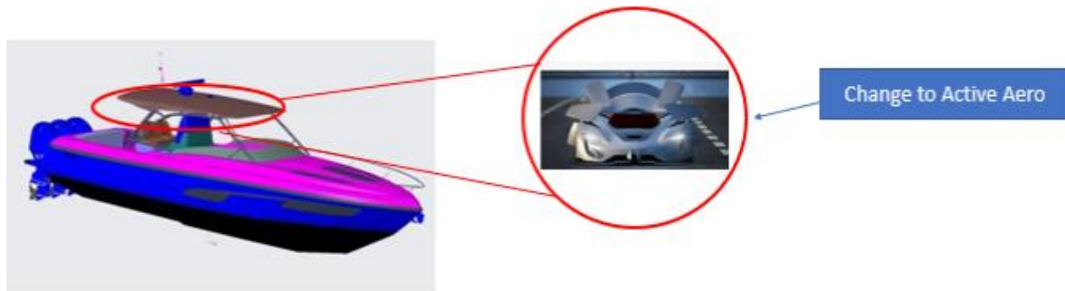
Figure 5: This design implements an active aerodynamics system to help generate lift and decrease drag. While lift generation is important for top speed, having increased drag will have a detrimental effect on performance. The active aero addresses both problems by changing shape to produce lift and changing shape to reduce drag.
